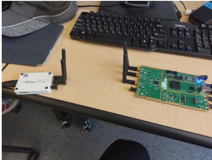
Figure 8. Ettus B210 and Ettus B205mini Connection to Antennas
